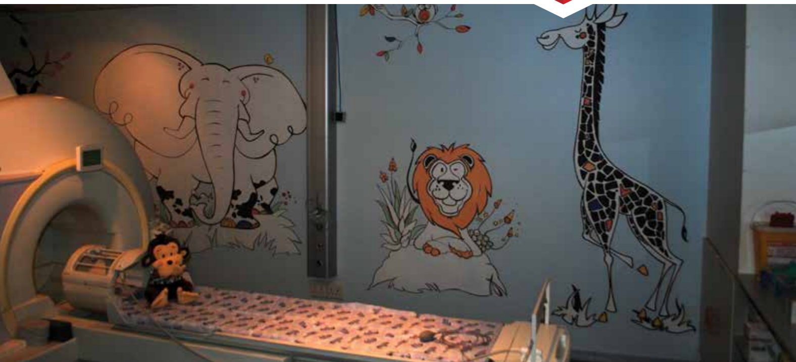
The Siemens 3 Tesla Magnetom Allegra is a compact, dedicated brain MRI scanner.
